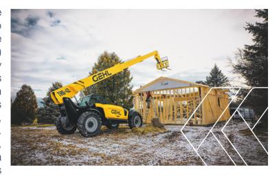
been completely redesigned with a new cab, providing enhanced comfort and better visibility around the machine and on the attachment. Noise pollution is greatly reduced to 80 dBA inside the cab. In the driver's cab, an intuitive dashboard provides operating and maintenance alerts, and the JSM (joystick switch and move) allows fingertip control of every function. For enhanced comfort and safety, this range also features an automatic parking brake.
