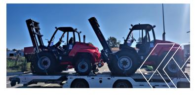
M40 model, presented at Conexpo, has a load capacity of 8,800 lbs, for two lifting heights of 22 feet with the triplex mast version, and 15 feet with the duplex mast version. This range is particularly suited to residential construction, public works or road infrastructures, as well as container handling in port areas.
