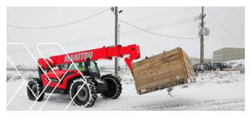
Steve Kiskunas, US Telehandler Product Line Manager, explains: "We have done a great deal of work on the comfort and performance of this new range. The new load-sensing hydraulic system improves smoothness and accuracy, and the combined hydraulic movements provide greater efficiency for increased productivity. The new transmission's automatic mode offers greater flexibility and optimum torque with less operator fatigue, with the option to switch to standard powershift transmission at any time."
