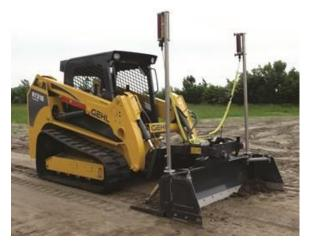
Gehl and Mustang brand machinery now have a **new dual-direction leveling bar.**
