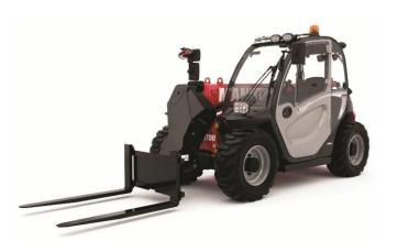
to the reduction of preventive and corrective maintenance costs, its ease of transportation, and high residual value. A wide selection of compatible attachments is available: waste grippers, box dumper, big bag handler, fork positioner, etc. The new MT 425 is therefore an ideal solution for outdoor handling (docks, quays, ports, and foundries) and for containers.
